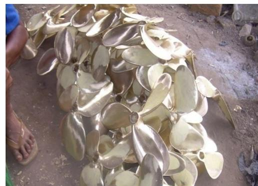
**Gambar 4.** Proses finishing hasil coran
